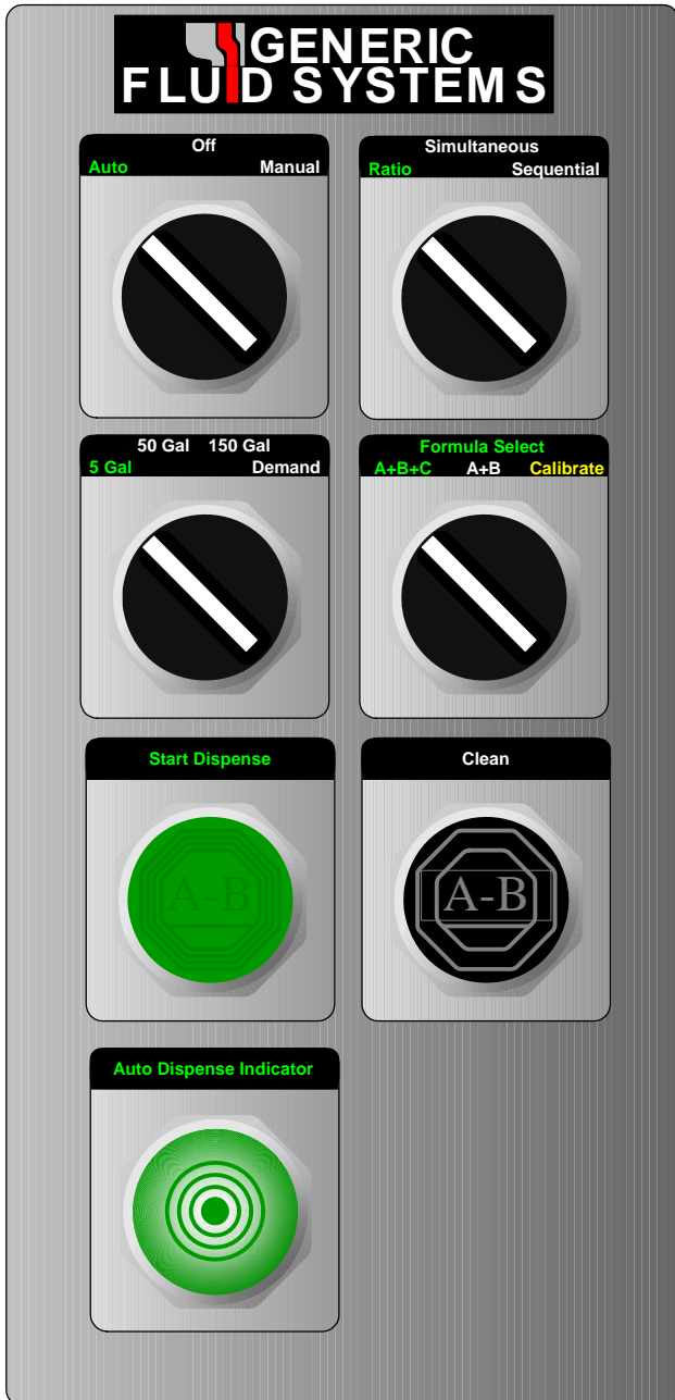
Operator Panel (Three-Ingredient Dispenser)
